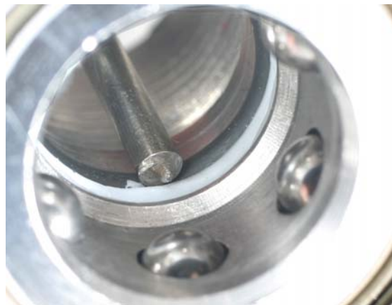
Figure 2: Use the smooth shaft of a small tool to work the O-ring and seal into place. The seal rests above the O-ring, nearer the spring-loaded ball bearings.
