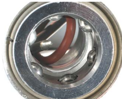
Figure 1: Use a machinist's scribe, a dental pick or a hand-fashioned tool to remove the existing O-ring and seal.
